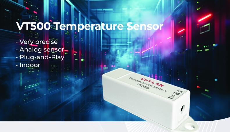
**VT500** Temperature sensor is an analog plug-and-play temperature sensor for indoor use only. Can be connected to any of the analog ports (A1...A8) of Vutlan monitoring systems. The accuracy of the sensor is  $\pm$  0.15 °C at room temperature. The maximum distance from the monitoring unit (or sensor extension unit) is 100 meters.
