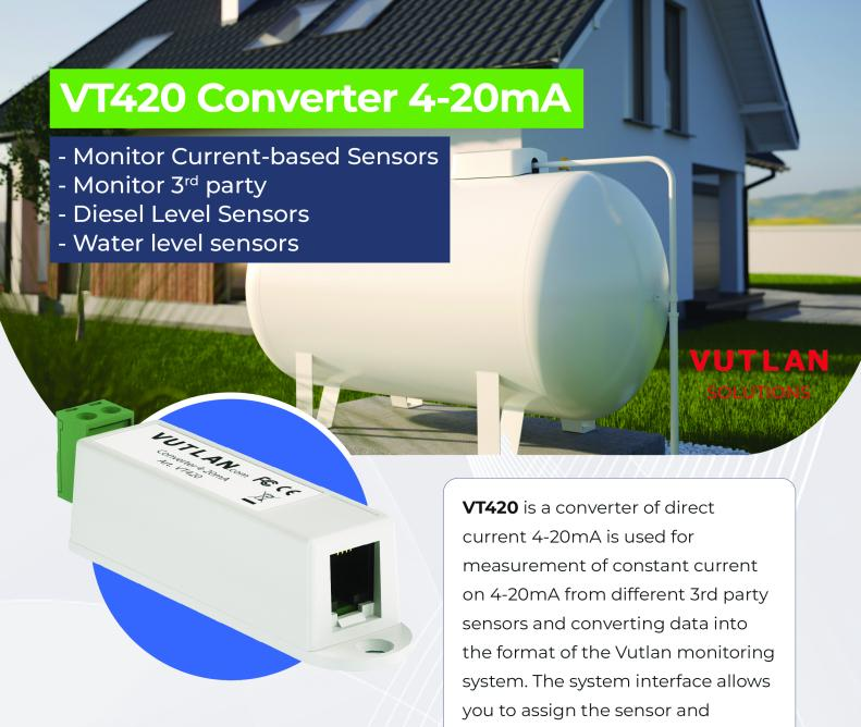
conversion. Operating temperature Device type Analog sensor, Plug&Play From -10° C to +80° C Current loop converter Operating humidity 5-95% (Non-Condensing) Usage 4-20 mA 60×18×18 mm Measured current Dimensions Galvanic 1 kV Accuracy 2% Isolation x1 RJ-12 / RJ-11 6p4c 100 mW Output **Power Consumption** 9030 33 100 **HS** Code Input Terminal 2P, pitch 5mm
